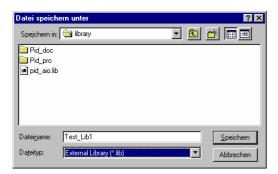
3. When saving the external library an additional header file is generated with the file name of the external library and the extension \*.h. This header file is the basis for the development of the C function.
