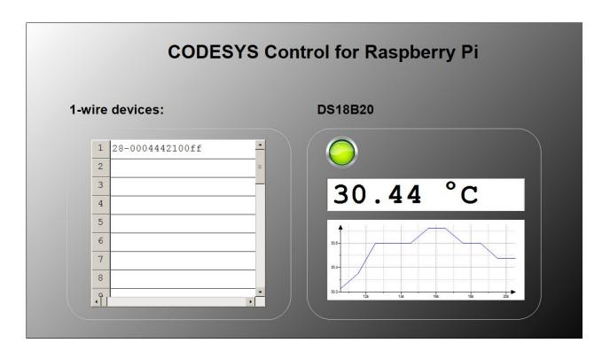
Note that the data exchange via 1-wire takes quite a lot of calculation time in this implementation, during which the task is blocked. Therefore it is recommended for time critical applications to assign the 1-wire devices to a task of low priority (see device configuration, tab I/O exchange, buscycle options).
