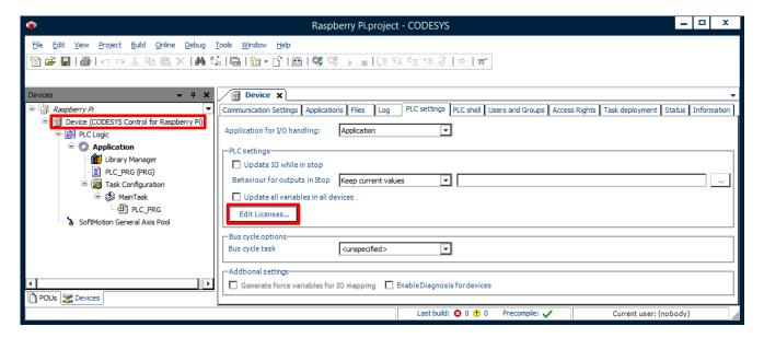
The licence activation is done under "Install licenses" / "Activate license" by entering the ticket number and transfer of the licence to the CODESYS Software Key (Softcontainer).
