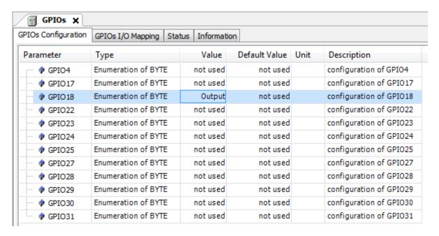
The inputs and outputs are available as DWORD in the tab "GPIOs I/O Mapping". Bit <X> of the DWORD correlates with GPIO <X>.
